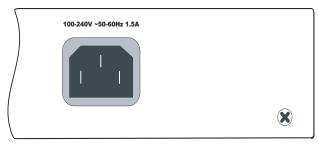
Figure 1-4 Power Supply Socket
